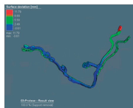
Figure 2: Distortion of a Craniomaxillofacial after the print in comparison to the initial geometry
