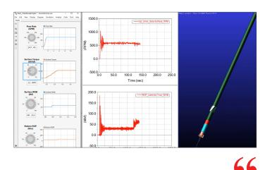
The comprehensive application being developed allows users to vary the drill string components, operating parameters, wellbore geometry, lithology and control algorithms being used to understand the effect on drilling dynamics.
