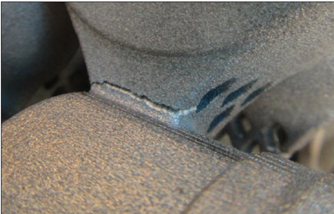
Figure 2: Example of macro-cracks on LBM parts that appeared during the manufacturing process due to part distortion and Simufact Additive stress predictions of the parts (Red is high, blue is low)
