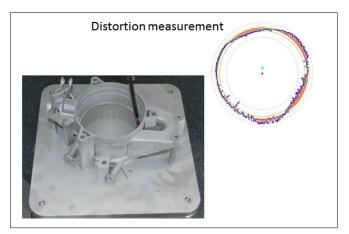
Figure 1 B: Measurement of the distortion at the top of the part
