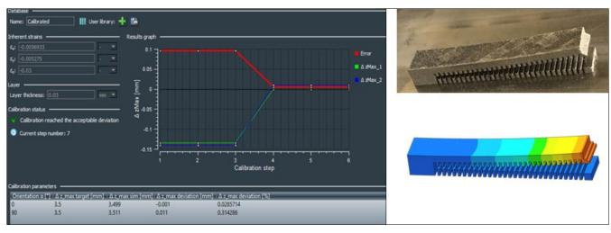
Figure 2: Calibration of inherent strains
