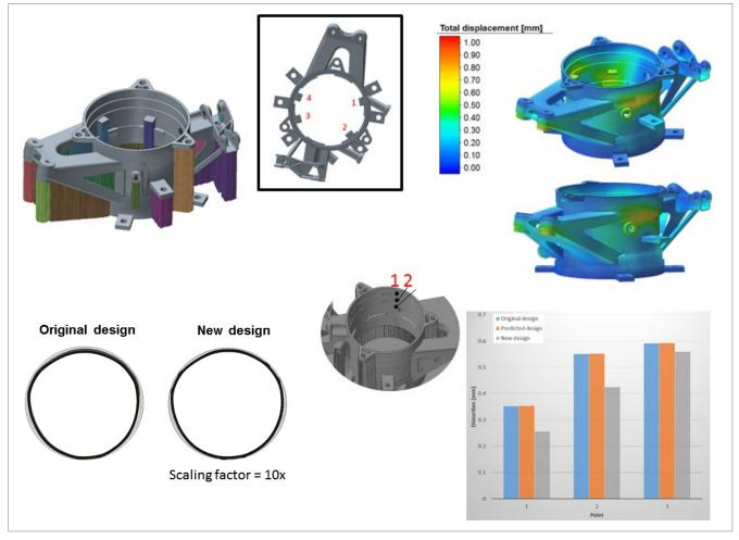
Figure 5: Simulation results of optimized part. A- New design, B- Distortion, C- Shape of the part with scaling factor 10x, D- Comparison of distortion values
