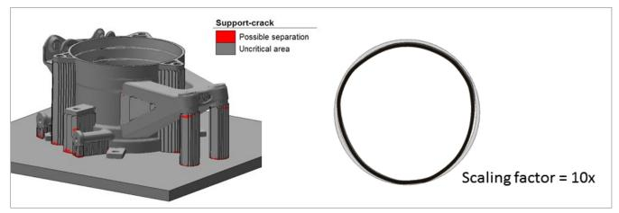
Figure 4: Simulation results with calibrated inherent strains. A- fracture areas, B- Shape of the part with scaling factor 10x
