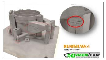
Figure 1 A: Printed wheel carrier. Separation observed in the support structure
