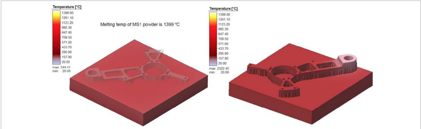
1. Melting temperature of 1399°C is ensured throughout the simulation process to avoid the thermal issues.
