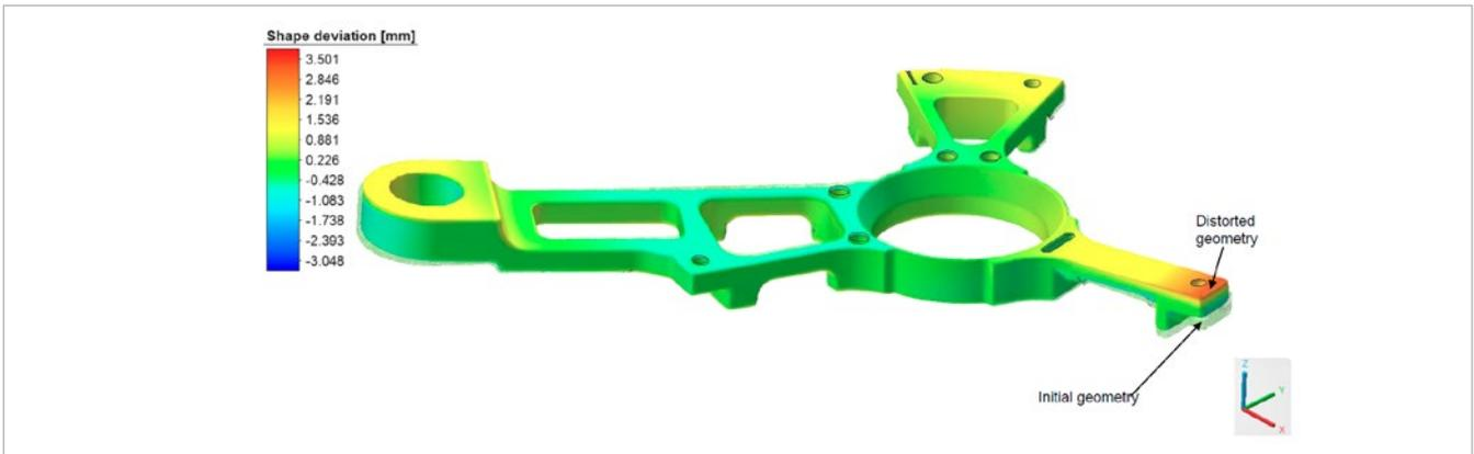
2. Final part distortion running out of tolerances, exceeding 3.5 mm
