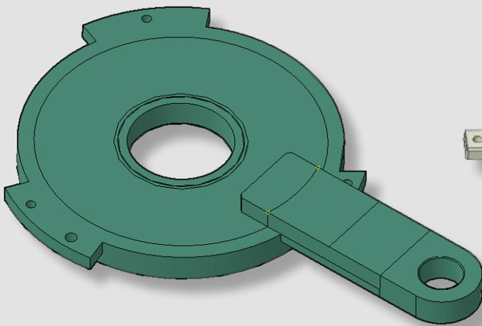
Traditionally (casted) manufactured fixture tool component
