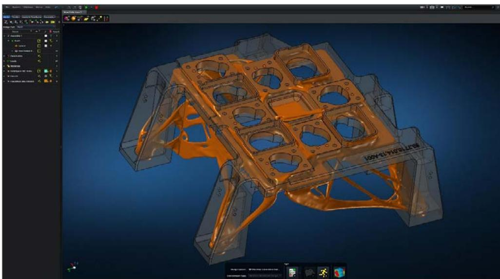
Comparison of a design variant with the original design in MSC Apex Generative Design
