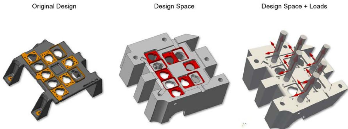
The existing conventional design was divided into design and non-design areas and was provided with loads in preparation for optimisation with MSC Apex Generative Design.
