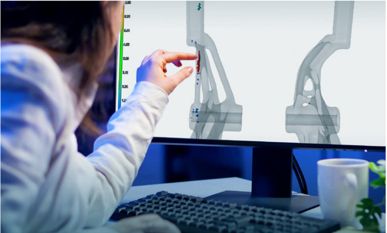
Figure 7: There are some pores in one of the legs of the component. However, an analysis by VGSTUDIO MAX shows no impact on the application when under load
