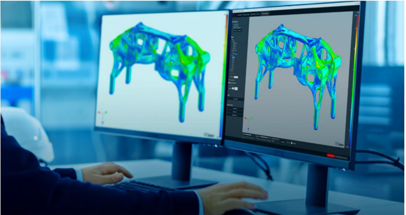
Figure 4: Manufacturing simulation of plastic printed parts avoids excessive deformation for maximum accuracy in the demanding gripper use
