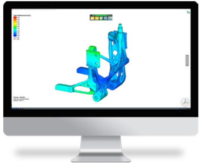
Figure 5: With Simufact Additive, metal-based production can be simulated in advance. The positioning, support structures and manufacturing parameters can thus be optimised and distortion and high stresses can be avoided.
