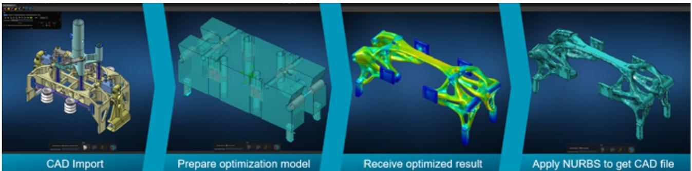
Figure 1: From CAD import for preparation of the model to CAD export for validation with MSC Nastran, optimisations can be implemented quickly and completely in MSC Apex Generative Design.
