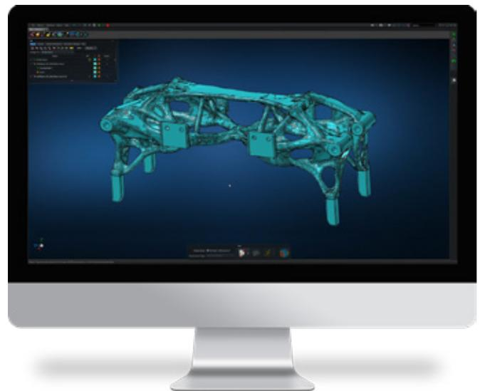
Figure 3: A retransition to standard CAD formats based on NURBS can be achieved at the touch of a button, even with complex structures
