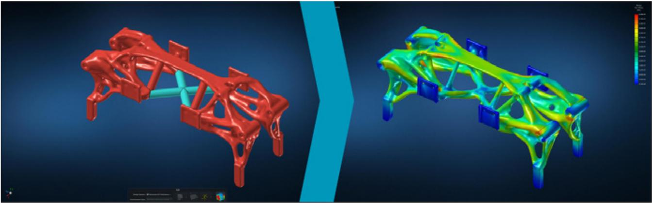
Figure 2: Subsequent changes can be inserted quickly with the geometry tools and then connected cleanly and meaningfully with just a few optimisation iterations.
