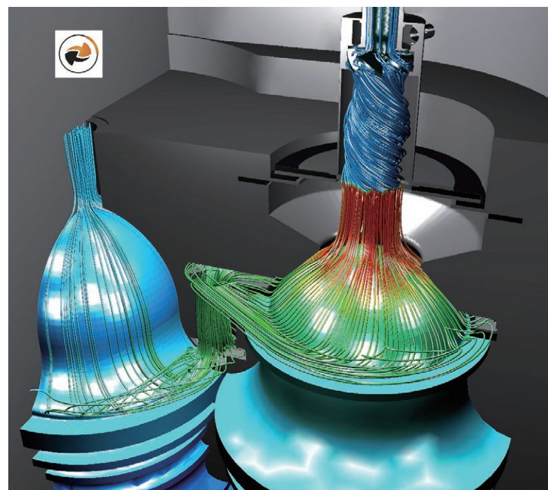
Figure 4: scFLOW predicted CFD flow lines and pressure drop inside the BoostHEAT boiler
