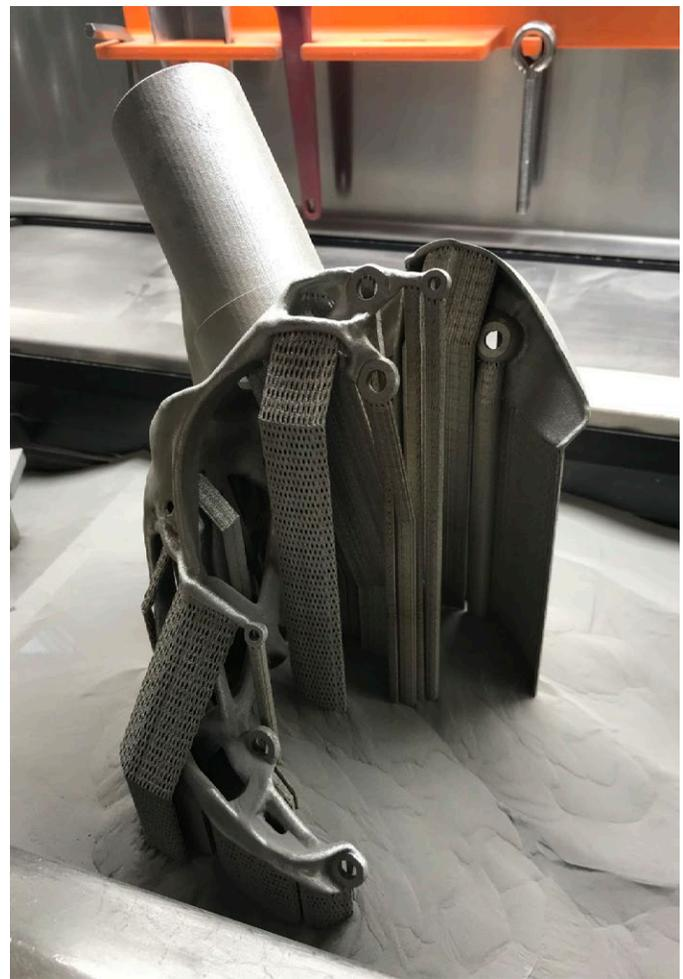
Figure 2: The motor mount was manufactured using the powder based SLM (selective laser melting) process. The support structures required for the process can be easily removed so that the ready-to-install solution is immediately available.
