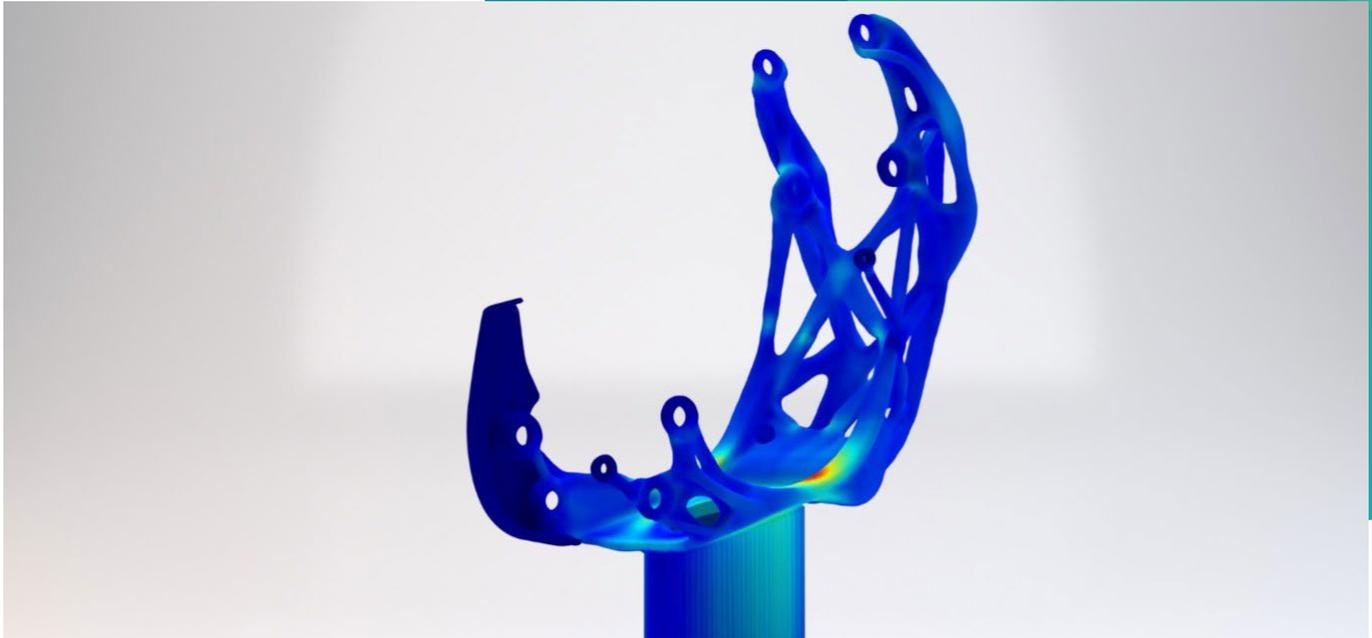
Figure 1: The simulation result shows homogeneous stress distribution in the entire component with very uniform colour distribution (blue/turquoise) and few critical areas (red).
