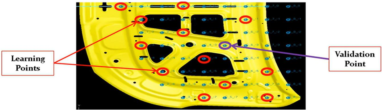
Fig 1: Location points to determine the injury score. Each location point listed has X&Y coordinates to the latch and the hinge, and the surface hardness.
