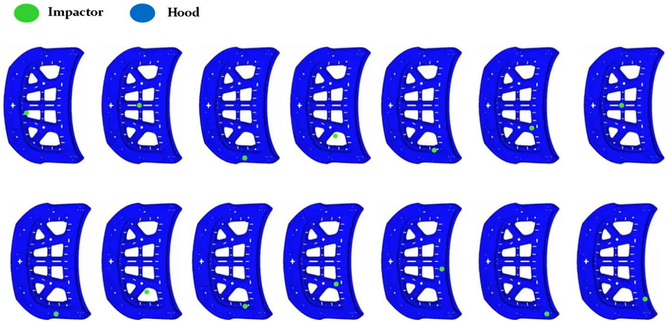
Fig 3: The 12 learning simulations used for ODYSSEE A-Eye. The placement of the green circle indicates the location of the head impact.
