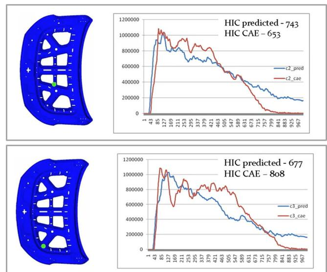
Fig 2: Acceleration curves for head impact on hood at two locations. Blue graph curve shows ODYSSEE A-Eye prediction, the red curve shows the FEM validation curve.
