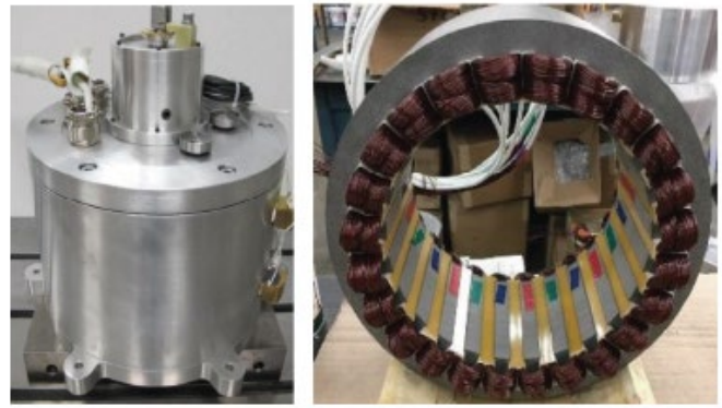
Figure 5 24/16 switched reluctance motor for a traction hybrid electric vehicle (HEV) application, designed by the researchers in the Canada Excellence Research Chair (CERC) in Hybrid Powertrain Program
