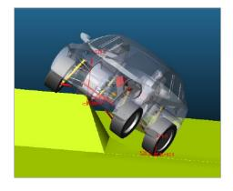
**Roll-stability events:** Ensure the safety and stability of the vehicle with roll-over simulations
