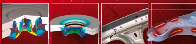
Self Piercing Riveting ... Clinching ... Adhesive Bonding ...
