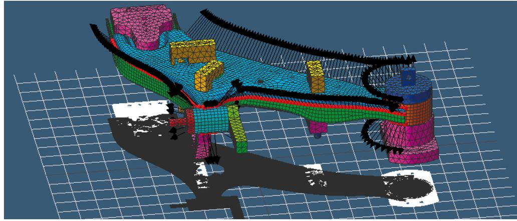
Case 1: Weld seam of swing arm is cracked, welding residual deformation is too large at key joining point
