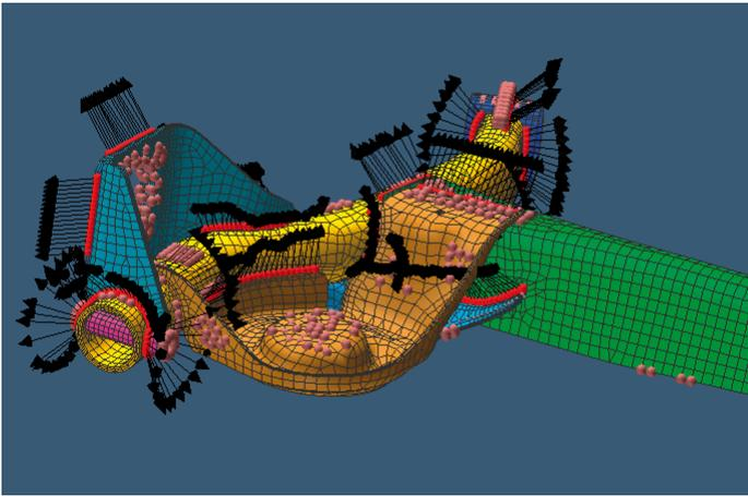
Case 2: Cracking of weld seam of torsion beam
